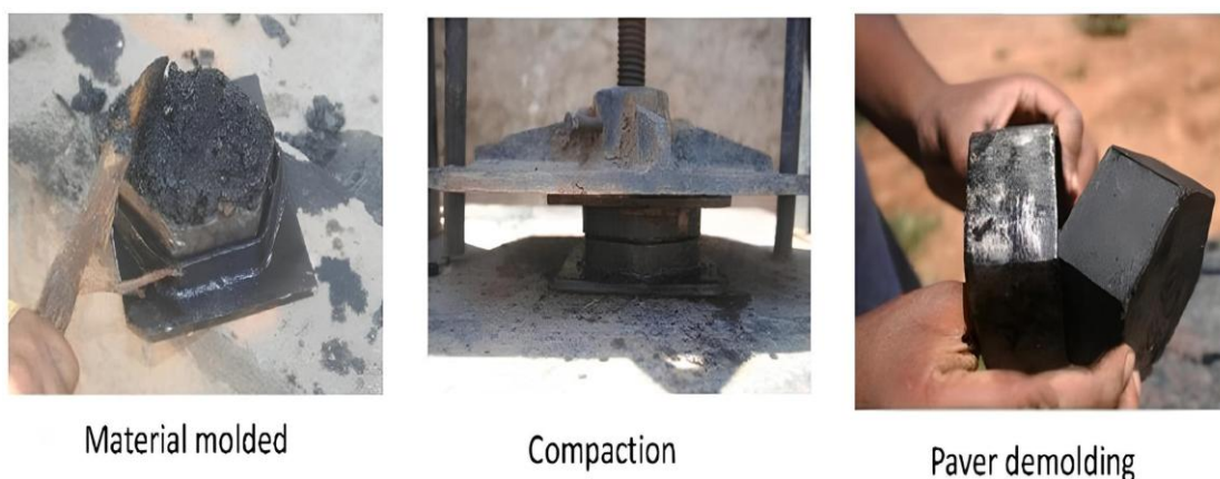
Figure 3. Process of producing paving blocks from plastic waste [5].
