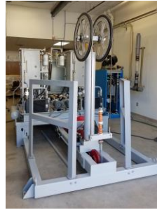
Figure 2 - Hydraulically driven demonstration rod pump
