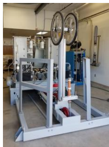
Figure 2 - Hydraulically driven demonstration rod pump
